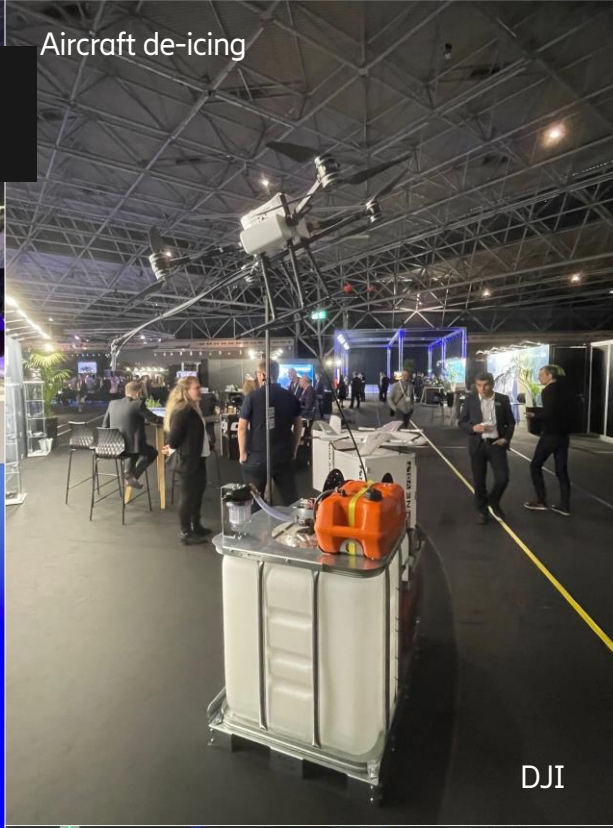
UAV able to lift 100 kg
